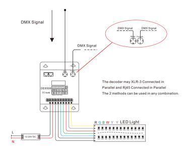
An amplifier is needed when more than 32 decoders are connected signal amplification should not be more than 4 times continuously DMX5000 output and DE8506's transmission lines can't be over 300 meters.
